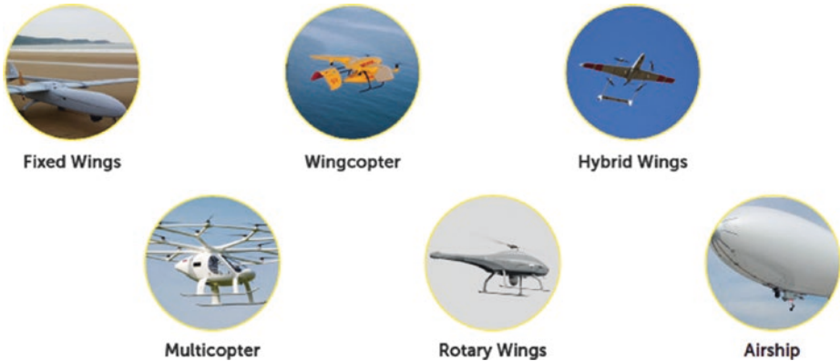
■ Fig. 16.2 Type of wing arrangements. (Author's own figure)
