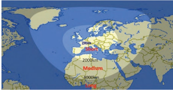
■ Fig. 6.12 Ranges short, medium and long around Zurich. (Great Circle Mapper, n.d.)
