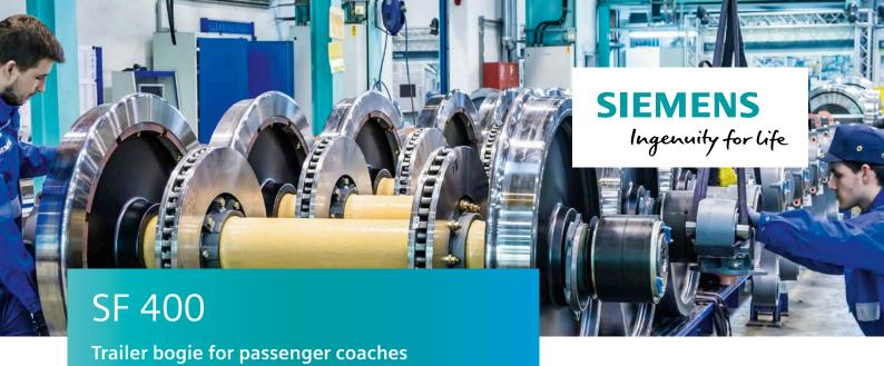
The bogie SF 400 was designed for push-pull service in locomotive-hauled passenger coaches. The maximum operational speed is 280 km/h.
