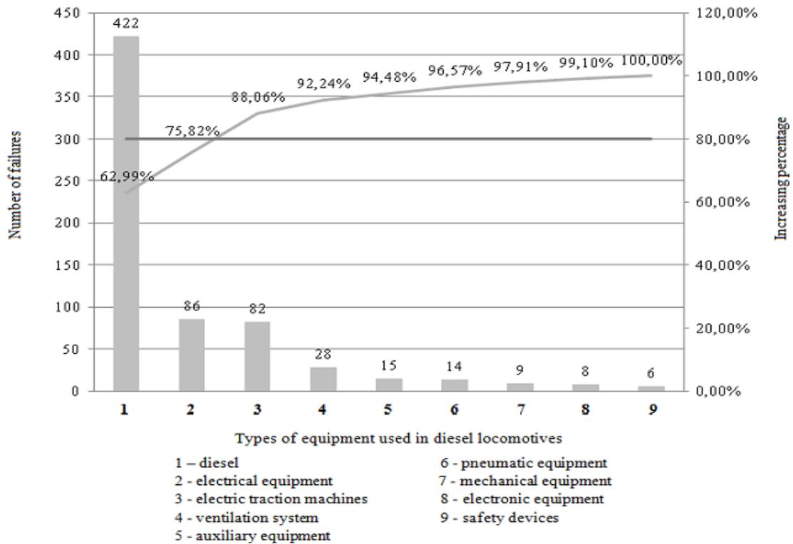
Figure 2. Distribution of cases of failures for 2017.
