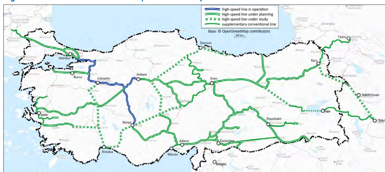
Figure III–24 Status of HSR network planned in Turkey
